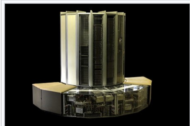
Cray-1 with internals exposed at EPFL
